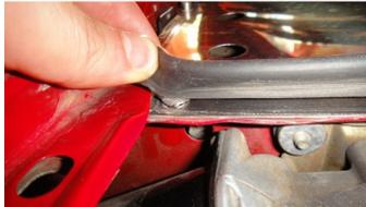
The clips need to be exchanged in the next step with the provided flat head bolts.
