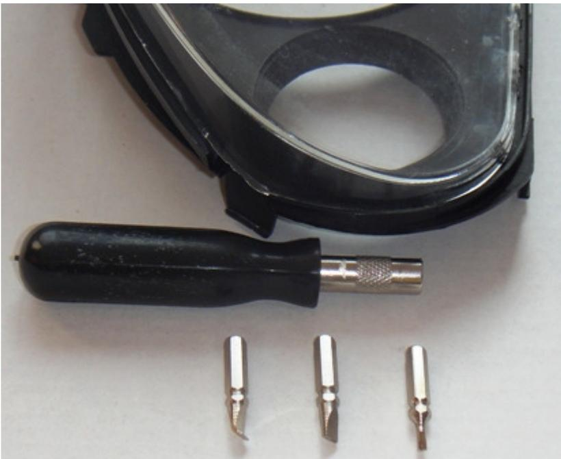
Please keep in mind that patience is essential. You need to be careful and gentle applying the force equally. If possible, try to heat up the part where you are working. Best to start is on the side. Try to lift by putting the screwdriver in the opened split, then equally lift, by opening on both sides.
