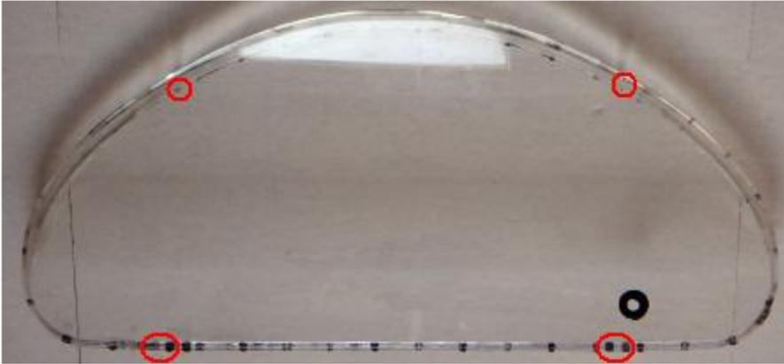
As next, you need to remove the rings off the body, as the panel attaches behind them. They are plastic that is glued with soft glue. Gently pulling them **equally** allows their removal, without being bend or destroyed.
