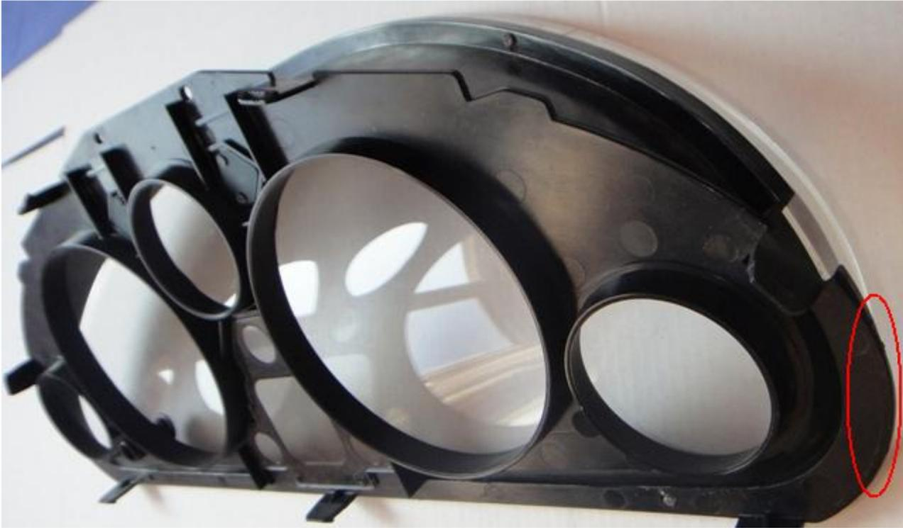
There are four pins on the glass that are glued to the body. You will most probably end up breaking them. Don't worry to crack the pins, instead of trying to save them, as they can potentially lead to a crack in the glass. It does not make any difference if they are broken or not, since you are going to glue the whole together.
