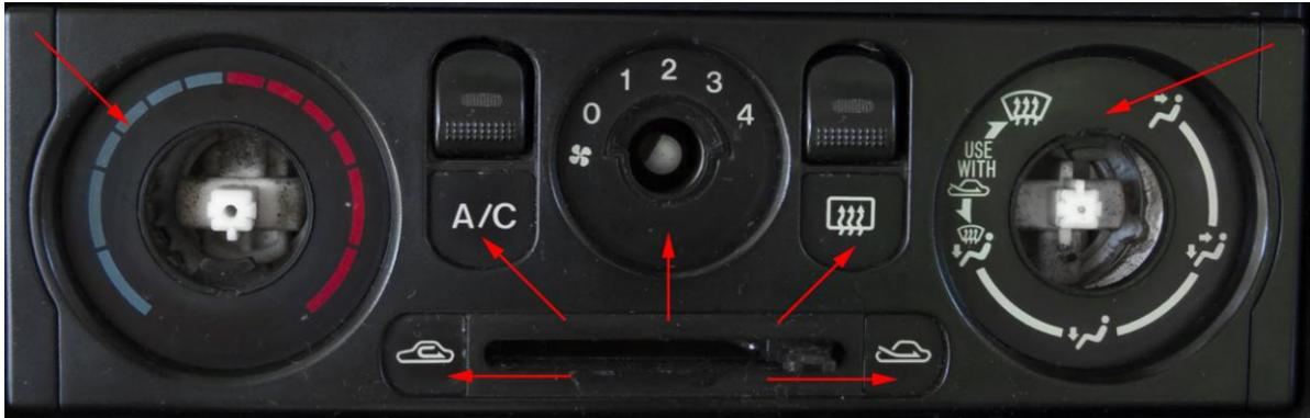
The plastic covers are glued to the heater panel. To remove them, you can use sharp utility knife/cutter and a small flat screwdriver. Gently slide the cutter along the edges until it is positioned below the plastic cover and carefully lift upwards.
