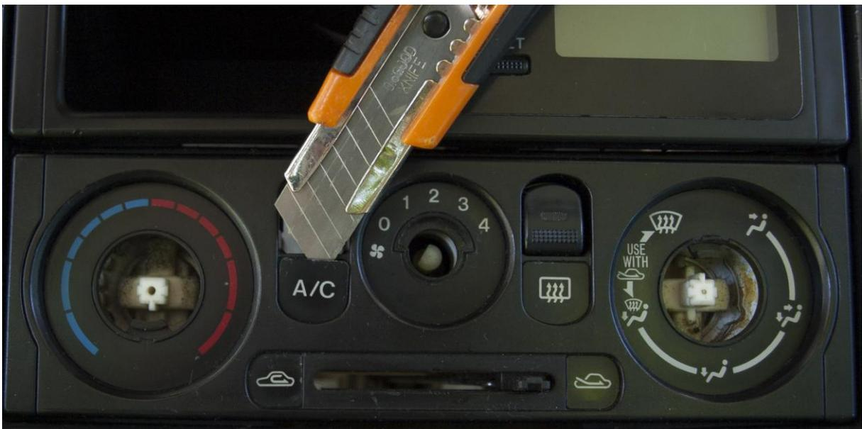
**Important:** After removing them, peel/clean the remaining glue. You can use a small flat screwdriver to peel the remains of the glue.
