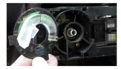
The labels panel has to be removed, it is held partly with glue.
