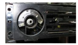
The stainless dial plate goes now in front of the original dial panel and covers it. Then it attaches back to its position at the front panel.
