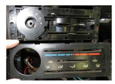
The transparent light guide has to be removed from the blower knob dial.
