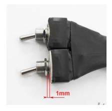
Mount the switches by pushing them through the cutouts of the brackets, placing the Hazard Switch Plate and tightening them with the knurled nuts. When tightened, the knurled nuts should be zeroed with the top side of the switches.
