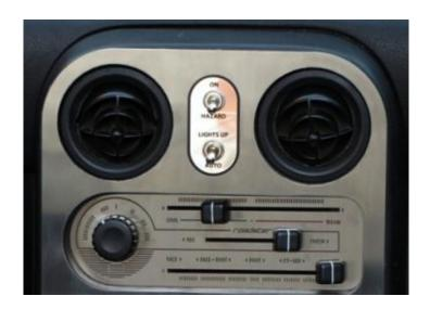
Stainless vintage style panel with toggle switches for the hazard switch and retractable headlights lock switch.
