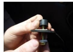
6. Now with the last screw, again place a white shim onto the screw, then through the door pull and door pocket hole, but again, do not fully tighten.
