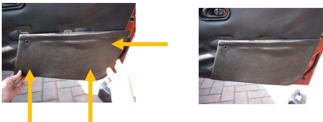
3. Insert the screw that is hidden in the pocket, but do not fully tighten this just yet.
